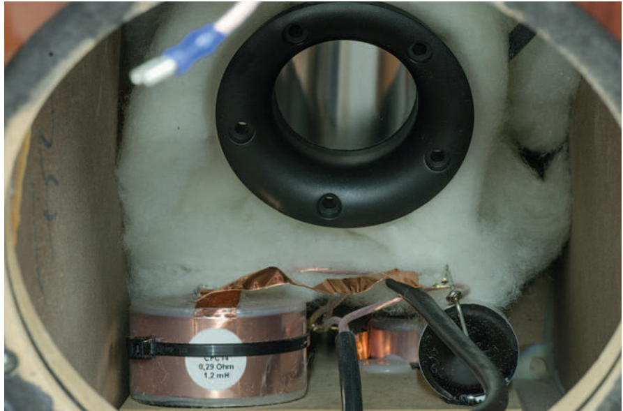
Looking through the midwoofer aperture reveals the crossover's point-to-point construction and the exceptional quality of the components employed, including copper-foil inductors and oil-impregnated capacitors. The driver rebate in the front baffle also reveals the sandwich construction of the cabinet panel, comprising two HDF layers bonded by an intermediate viscoelastic material.
