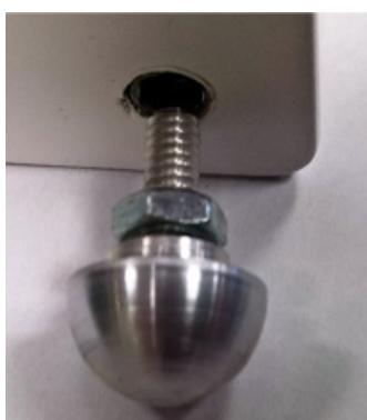
**The base of the cabinet is fitted with a machined  $\frac{1}{4}$ " 20 thread insert to accommodate the decouplers.**
