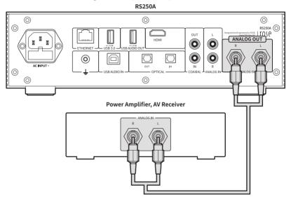
⚠ Caution: Before connecting the product to the power amplifier, set the volume to mute or below step 5 and then connect it using an RCA cable.
