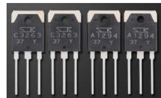
Bipolar transistor Current Capacity: 15A
