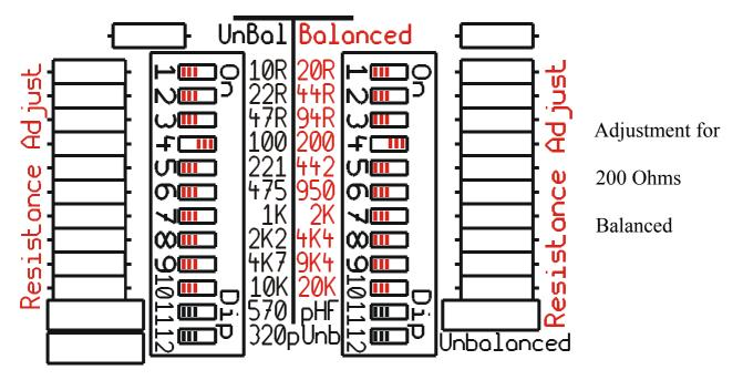
Possible adjustments on the left and right 12 fold DIP switches "Input Resistance" The following chart shows you on the left column the value you get when you switch On the Dip switches shown in the right columns.
