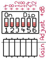
The gain can easily be adjusted on the 6 fold DIP switches "Gain Adjust". The switches can be combined to get higher gain.
