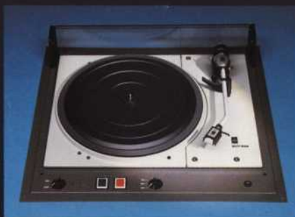
The photo shows the EMT 938 Broadcast Disk Reproducer with dust cover removed, installed using method B at the right.
