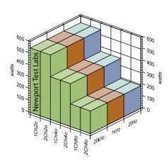
Power Output: Both channels driven into 8-ohm, 4-ohm and 2-ohm non-inductive loads at 20Hz, 1kHz and 20kHz. [Audio Analogue Maestro Anniversary Integrated Amplifier]
