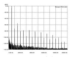
**Graph 3:** Total harmonic distortion (THD) at 1kHz at an output of 150-watts into an 8-ohm non-inductive load, referenced to OdB. [Audio Analogue Maestro Integrated Amplifier]
