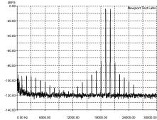
**Graph 5:** Intermodulation distortion (CCIF-IMD) using test signals at 19kHz and 20kHz, at an output of 1-watt into an 8-ohm non-inductive load, referenced to 0dB. [Audio Analogue Maestro Integrated Amplifier]
