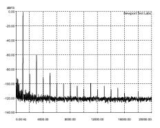
**Graph 2:** Total harmonic distortion (THD) at 1kHz at an output of 1-watt into a 4-ohmnon-inductive load, referenced to OdB. [Audio Analogue Maestro Integrated Amplifier]
