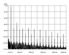
**Graph 4:** Total harmonic distortion (THD) at 1kHz at an output of 300-watts into a 4-ohm non-inductive load, referenced to OdB. [Audio Analogue Maestro Integrated Amplifier]
