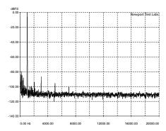
**Graph 1:** Total harmonic distortion (THD) at 1kHz at an output of 1-watt into an 8-ohm non-inductive load, referenced to OdB. [Audio Analogue Maestro Integrated Amplifier]
