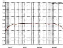
**Graph 6:** Frequency response of line input at an output of 1-watt into an 8-ohm non-inductive load (black trace) and into a combination resistive/inductive/capacitive load representative of a typical twoway loudspeaker system (red trace). [Audio Analogue Maestro Int. Amplifier]
