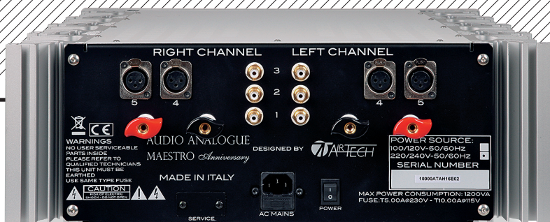
ABOVE: No MM/MC phono stage but the five line inputs include two balanced on XLRs. 'Propeller Post' 4mm speaker outlets feature substantial gold-plated terminals
