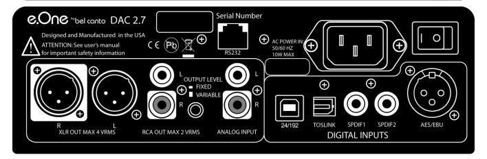
IMPORTANT: If using the DAC2.7 directly into a power amplifier, ensure that the Fixed/Variable Output button is in the OUT (variable) position. Operation in Fixed Mode directly into the amplifier could cause extreme output levels, clipping and damage to the loudspeakers, amplifiers or your ears!
