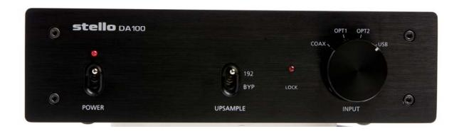
**POWER**: Turn the switch lever up to turn on the unit. Red LED will be on to indicate the DA100 is operating.
