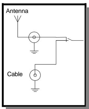
To enable FM stations to be received from either an external antenna or a cable feed, two antenna connections have been provided. The FM AGC automatically caters for the nominally higher strength signal associated with direct cable feeds, reducing them to a more suitable level for the T32R's FM front end.
