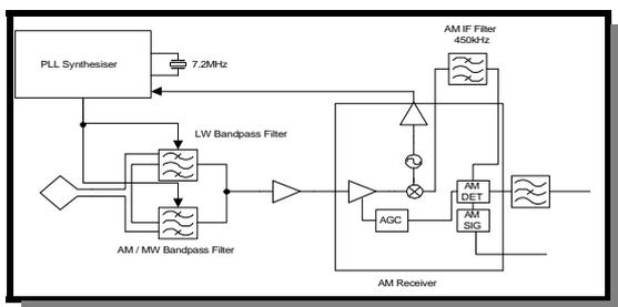
The mixer is driven by an automatic, level-controlled oscillator and the local oscillator output to the synthesiser is buffered to avoid strong signal interference (using a similar technique to the FM RF stage).
