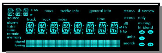
The custom display incorporates a dot matrix area for radio text messages and a larger 8 digit alphanumeric area for station names and tuning frequencies. Not content with the poor legibility of the standard “starburst” display, TAG McLaren Audio re-designed this font from first principles culminating in the TAG McLaren ‘Dot Burst’ font. This substantially increases the legibility of the display.
