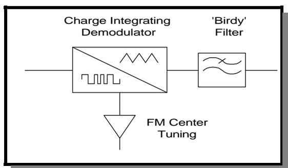
harmonics of the 38 kHz suppressed sub carrier of the encoded multiplexed stereo audio. These harmonics, if passed unchecked, are notorious for producing beat interference with adjacent channels which manifest themselves as unwanted tones or 'birdies'.
