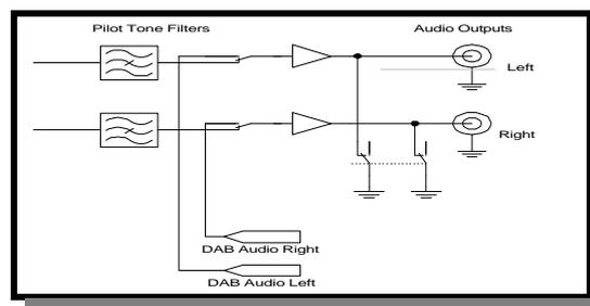
The analog stages, from the frequency to voltage demodulator, use precision, metal film, Vishay resistors. For ultimate fidelity muting is controlled by a relay which mutes the signal by shunting to 0 V to avoid relay contacts in the signal path.
