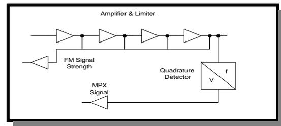
The amount of limiting applied, combined with the AGC at the RF front end, provides an accurate indication of the received signal strength. This is fed to an analog to digital converter onboard the microcontroller, which provides a display of the received signal strength on the custom Vacuum Fluorescent Display (VFD).
