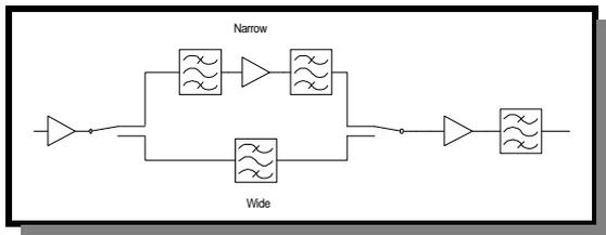
In 'wide' mode a Gaussian (flat group delay) filter provides minimum distortion with moderate selectivity. In situations where greater selectivity is required the 'narrow' mode selects an alternate filter path employing a two section Butterworth (maximally flat) filter.
