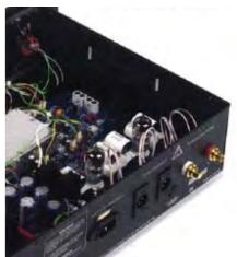
Onix tuners — have sported custom-designed tuner heads. The downside to this custom produced front end is the prohibitive cost. Magnum Dynalab's five-stage tuning front end is entirely custom made and must be one of the last tuners to do so. In the process, this means the method of holding onto a radio signal is now a combination of heavily-shielded toroidal transformer and stabilised power supplies.
