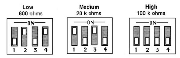
The "low" setting is for use with most direct-coupled solid-state preamplifiers such as those made by Jeff Rowland Design Group; the "medium" setting is for use with most solid-state, hybrid and some tube preamplifiers; the "high" setting is for use with most tube preamplifiers. We have provided these different settings so that you may find which one provides the best sonic results in your system. Your amp comes set from the factory at the "medium" (20 k ohms) adjustment.
