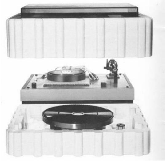
The arrangement of the packed turntable is shown in Figure 2. The upper styrofoam packing may easily be removed by grasping the opening on either side and lifting straight up.
