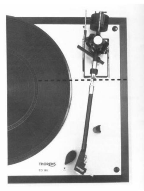
The TP 11 Mk III tone arm consists of the bearing assembly and the TP 63 cartridge wand, illustrated in Figure 7. The cartridge wand with pickup cartridge is plugged into the bearing assembly and secured by tightening the knurled collar. Instructions for mounting a pickup cartridge are given in Section VIII.
